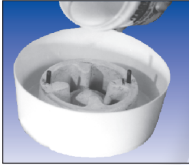
Pouring Replicast Around a Model
