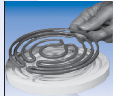
Placing Heater Coils in Insulating Disk
