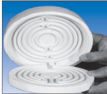
Removing 740 Insulating Plate From Mold
